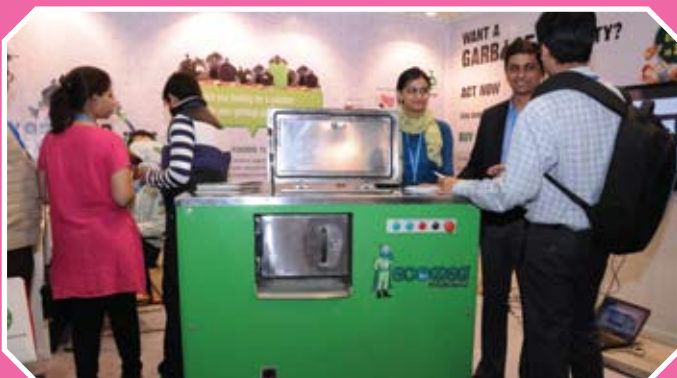
Ecoman Compost Machine from EcomanEnviro Solutions Pvt. Ltd. This machine produces compost from biodegradable in just 24 hours. Its best suited for building societies and apartment complexes.
