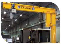
JIB CRANE CAPACITY: Up to 3.2 ton
