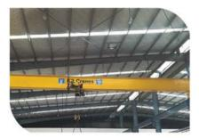
SINGLE GIRDER CRANE CAPACITY: Up to 15 ton
